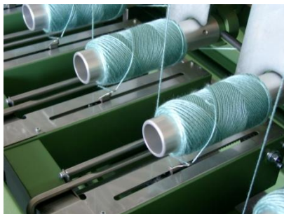
Fully-electronic traverse motion for precision thread laying
